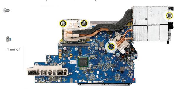
2. Tilt up the video card with attached heatsink, and disconnect it from the card connector on the logic board (as shown with the iMac (24-inch) video card.)
